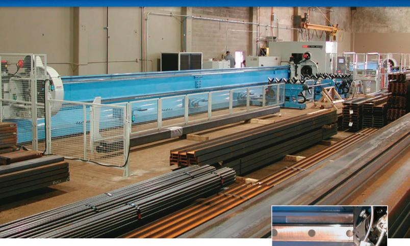
**Laser processing** of tube, pipe, bar, shapes, custom shapes and extrusions is a cost saving specialty of Farwest.
